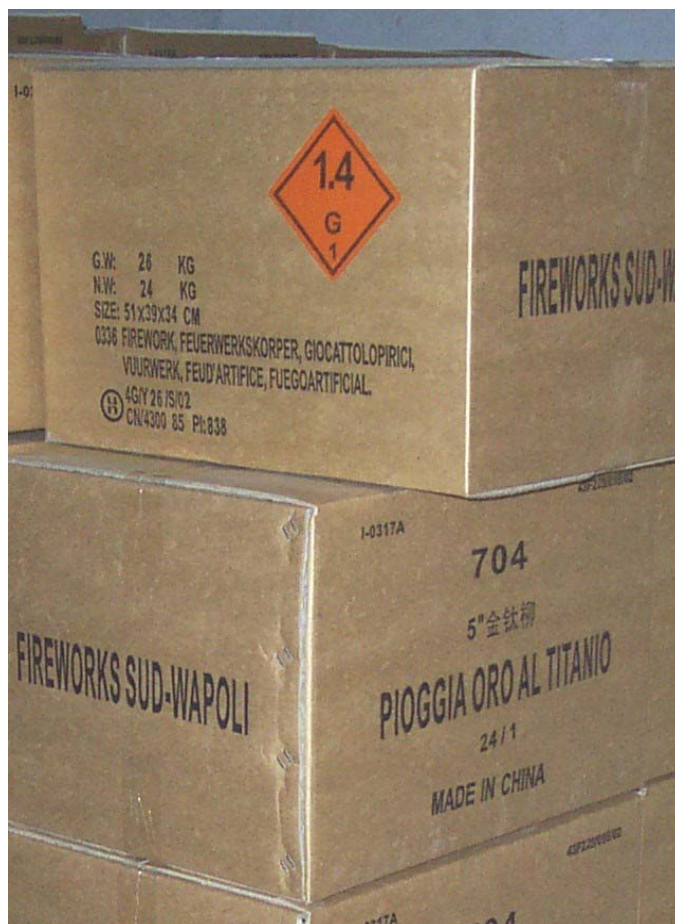
Photo 14. A warehouse full of 5” and 6” aerial fireworks shells in a Chinese warehouse await shipment to a European customer. Note the 1.4G classification and the various European language descriptions on the top carton of 5” aerial shells. These same aerial fireworks would be classified as 1.3G if shipped to the United States and other markets.
