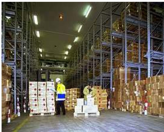
Photo 15. A distribution warehouse utilizing rack storage for imported 1.4G fireworks in Hamburg, Germany. No sprinkler system is apparent and the stacks of cartons on these pallets are not stabilized. Electrical systems do not appear to be explosion proof and motorized equipment is clearly used to move the pallets of fireworks. Distances from this building to other buildings and public areas is not known.
