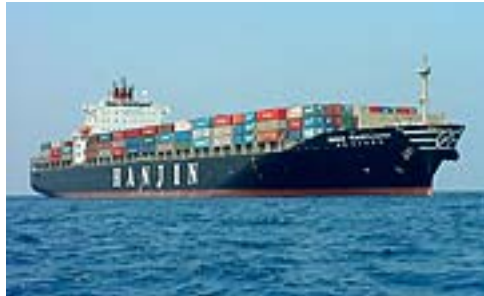
Photo 1. The newly built M/V HANJIN PENNSYLVANIA (starboard) fully loaded with containers. Holds one-six are from the bow to the accommodation, holds seven and eight are from the accommodation to the stern. Note how high in the water the ship is in this picture.
