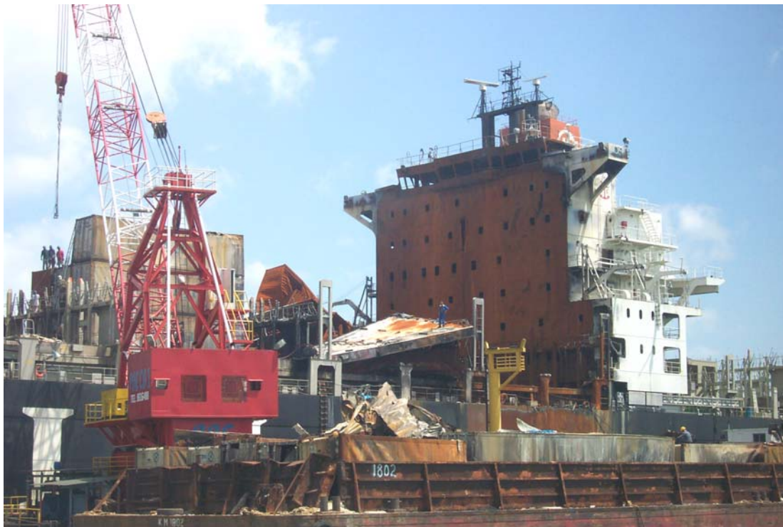
Photo 11. The M/V HANJIN PENNSYLVANIA (port) in Singapore during salvage and recovery operations. Note the twisted and upraised deck hatch now resting in the port side forward rack above hold six. The deck hatches from the port side and center racks in the aft rack of hold six are missing.
