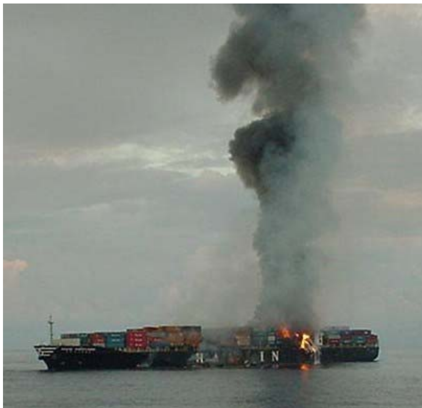
Photo 6. The M/V HANJIN PENNSYLVANIA (port) after the explosion of Nov 15 th in hold six. Fires continue to burn above hold six and smolder above hold four. Note the missing containers above hold four and the plume of gray-black smoke from hold six.
